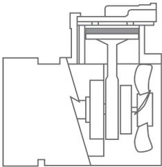
In a reciprocating motion, a flexible cup mounted on top of the connecting rod creates vacuum or pressure as the cup maintains a seal against the cylinder walls in a rocking motion.
